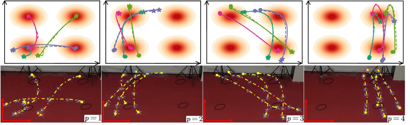
Fig. 5. The hardware experiment of ESPC with  $N = 4$  and  $N_p = 4$ . In Row 1, the solid and dashed lines represent the planned reference trajectories and the actual trajectories. Row 2 shows the trajectories of the quadrotors.
