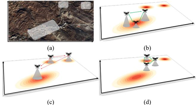
Fig. 1. A motivating example. (a): Mountainous area with three regions to be searched. (b): Drones are connected while gathering information. (c): Drones disconnect to gather information in different regions. (d): Drones reconnect to share the collected information. The planner needs to handle both connectivity maintenance and information gathering.
